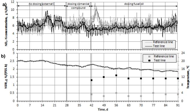
**Figure 1.** Results of the full-scale experiment at the Gdynia WWTP: (a) behaviour of  $NO_3$ -N in the test and reference lines (the bold lines represent moving averages with the period of 1 d), (b) process temperature and the NURs determined under laboratory conditions for the mixed liquor from the test line (with dosing fusel oil) and reference line (without dosing fusel oil).
