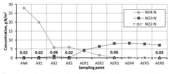
**Figure 1.** Measured concentration profiles of N species inside the bioreactor at the Gdansk WWTP (ANA- anaerobic zone, AX – anoxic zone, AER – aerobic zone).
