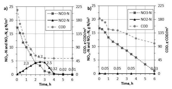
**Figure 3**. Sample results of the one-phase experiments with the settled wastewater (a) and fusel oil (b) in the lab-scale batch reactors (non-acclimated biomass)
