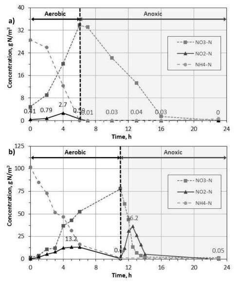
**Figure 4.** Sample behaviour of N species (NH<sub>4</sub>-N, NO<sub>3</sub>-N and NO<sub>2</sub>-N) during acclimation of the process biomass to ethanol during reject water treatment: (a) non-acclimated biomass, (b) 4-week acclimation
