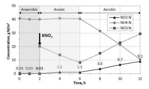
Figure 2. Measured concentrations of N species during a sample 3-phase batch experiment with the mixed liquor and settled wastewater at the Gdansk WWTP
