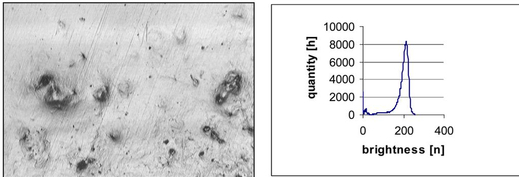
**Fig. 2.** Eroded surface and its histogram used to define level of blackening ( $z$ )
