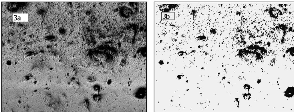
**Fig. 3.** Surface of steel 45 deformed by cavitation impingement after 14 min of cavitation attack. 1a – monochromatic picture, 1b – the same picture registered at the binarisation threshold 40. Upper part of the photo refers to the unremelted zone of the material and the lower part comprises the zone treated with laser beam
