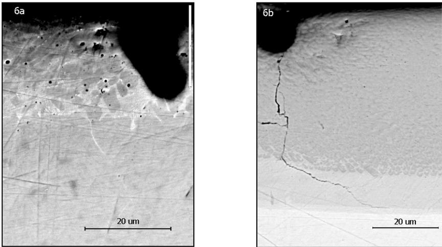
Fig. 6. Cavitation pits on the steel 45 surface alloyed with niobium (fig. 6a) and with FeCr+SiC powders (fig. 6b)
