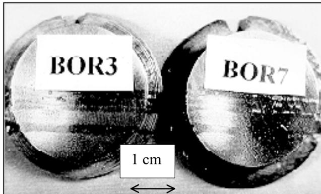
Fig. 1. View of the samples after 38 minutes exposition to cavitation attack
