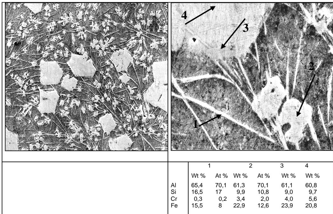
Fig. 5. SEM micrograph and chemical composition of the precipitates of the Al-Si hypoeutectic alloy obtained by chemical reaction of chromium steel stirrer with liquid alloy while stirring for 60 minutes
