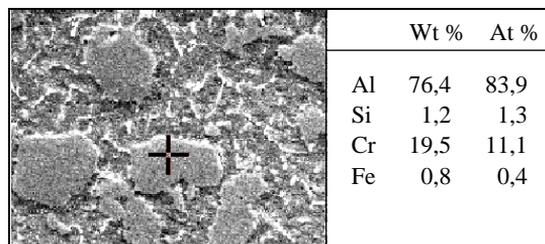
**Fig. 2.** SEM micrograph and the approximate chemical composition of the particle (marked +) of the same sample as in Fig. 1a. Magnification 500x
