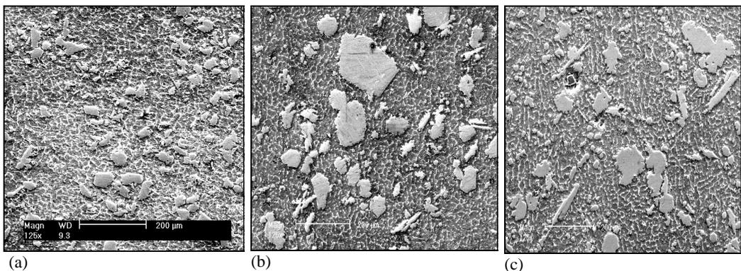
**Fig. 1.** SEM micrographs of eutectic Al-Si matrix composites after incorporation of: a) Cr powder, b) Cr+Fe powders and stirring 30 minutes, c) 120 minutes. Magnification 125x
