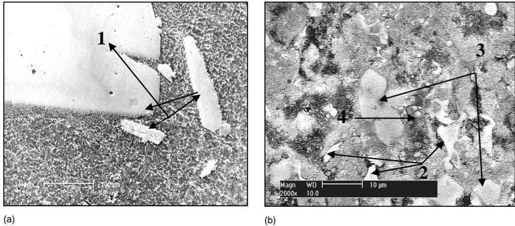
**Fig. 3.** Macrograph of the structure of the alloy obtained by mixing the eutectic Al-Si alloy with chromium steel scraps and stirring for 60 minutes (a) Magnification 125x, (b) new precipitates of Al, Fe, Cr, Si at magnification 2000x
