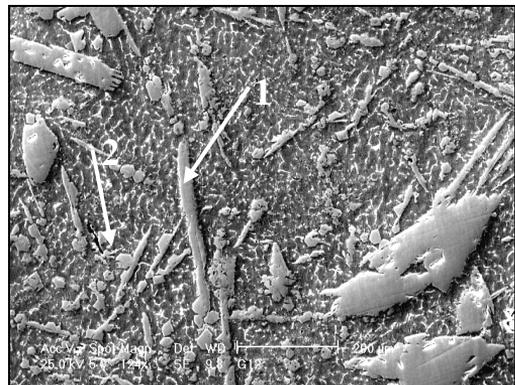
**Fig. 4.** SEM micrograph of the eutectic Al-Si matrix composites obtained by chemical reaction of the stirrer and liquid alloy after stirring for: a) 60 minutes, b) 90 minutes
