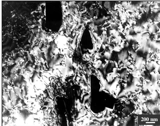
Fig. 14. Precipitate and cellular dislocation structure at intensity equal  $J = 5.13 \text{ mW/m}^2$
