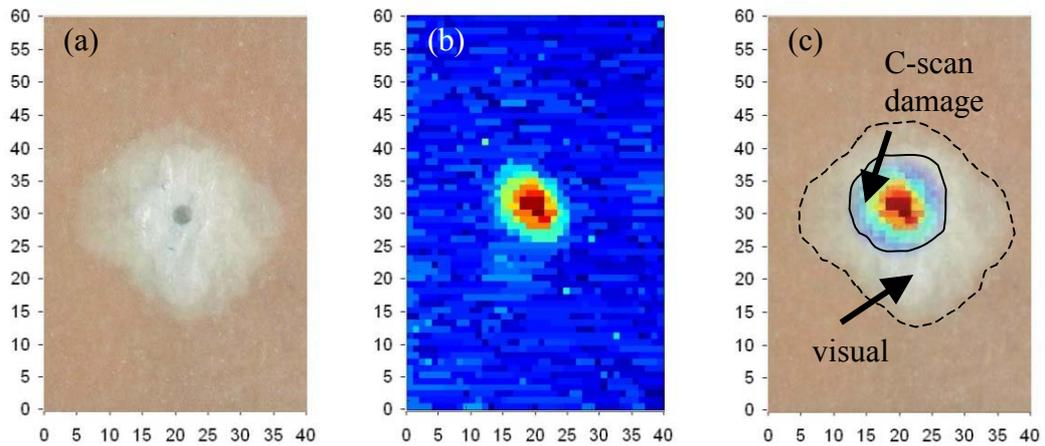
**Fig. 5.** Comparison of visual (a) and C-scan areas of damage (b) in “pinkglue” specimen subjected to impact 19,7J. Comparison (c).
