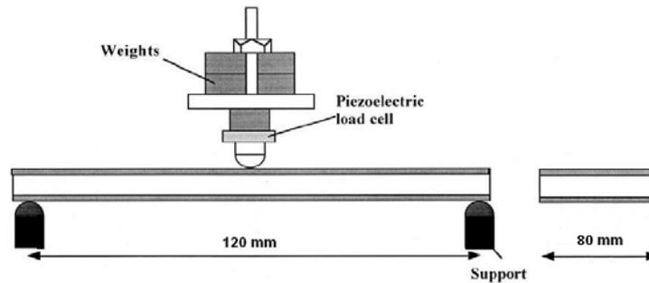
**Fig. 1.** Schematic diagram of impact conditions.
