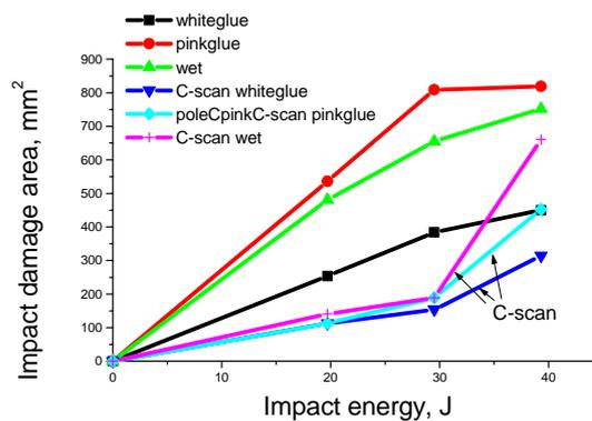
**Fig. 6.** Impact damage area as a function of impact energy for three types of sandwich structures: visual inspection and C-scan results.
