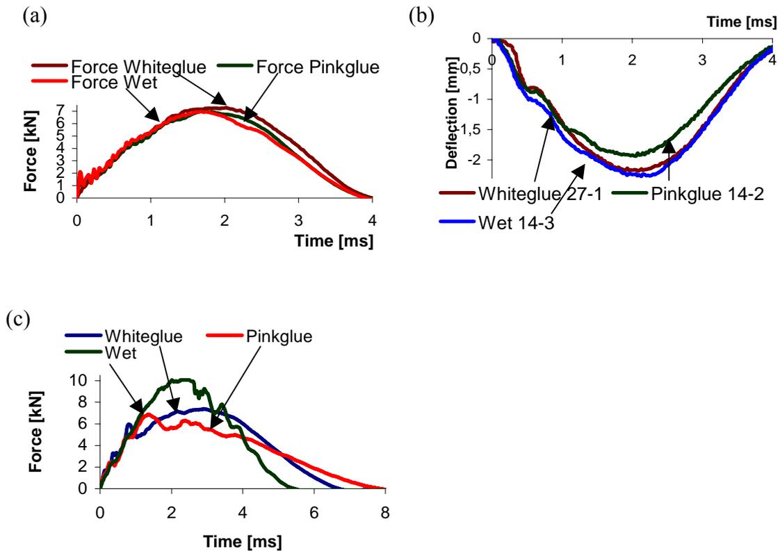
**Fig. 2.** Load (a), deflection (b)-time characteristics showing the response of the 3 different sandwich samples under impact 39,3J, (c) load-time plot for 51,6J (core crack in “pinkglue” and “whiteglue” samples).
