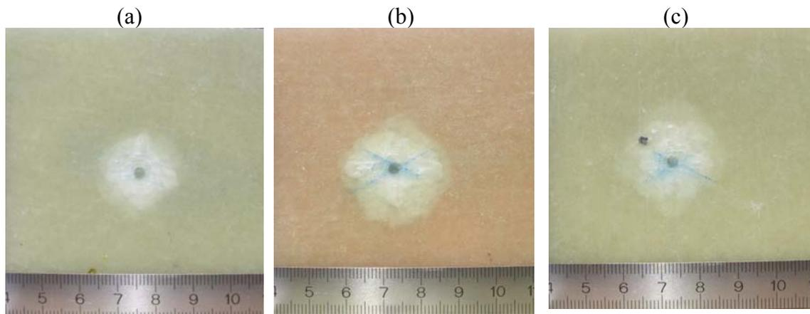
**Fig. 3.** Illustration of damage observed visually on the surface of the samples subjected to impact 19,7J: (a) “whiteglue”, (b) “pinkglue”, (c) “wet” sample.
