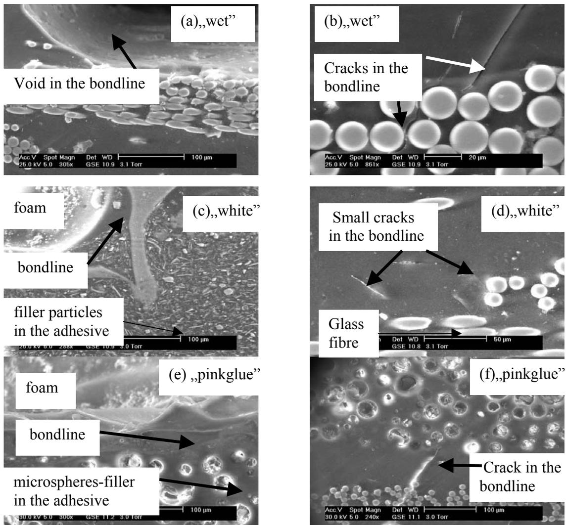
Fig. 8. Face/core interfacial area prior to impact (a,c,e), and after impact 19,7J (b,d,f), “wet”, (a,b), “whiteglue”, (c,d), “pinkglue” (e,f).
