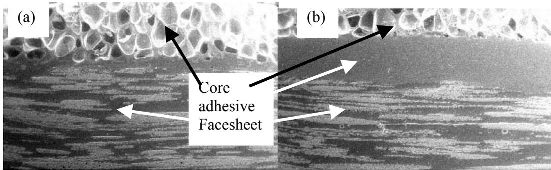
Fig. 7. Macroscopic view of the sandwich structure “wet”(a), “whiteglue” (b) sample.
