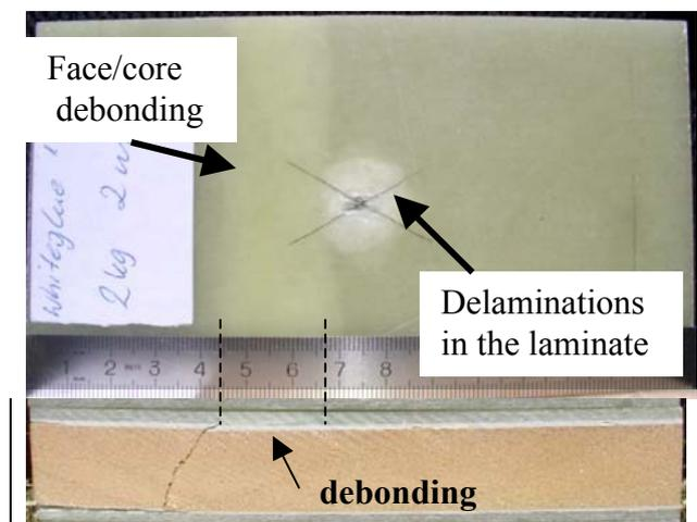
**Fig. 4.** Core-crack damage observed on the surface and cross-section of the laminate.
