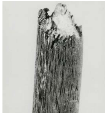
Fig. 3. Surface and fracture area for AlZn5Mg1 alloy of the T6 1 temper after stress corrosion test for 50 h at +100 mV vs. E_{cor}
