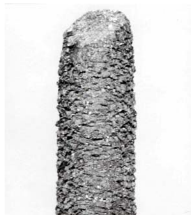
Fig. 1. Surface and fracture area for AlMg4.5Mn alloy after stress corrosion test for 100 h at +100 mV vs. E_{cor}
