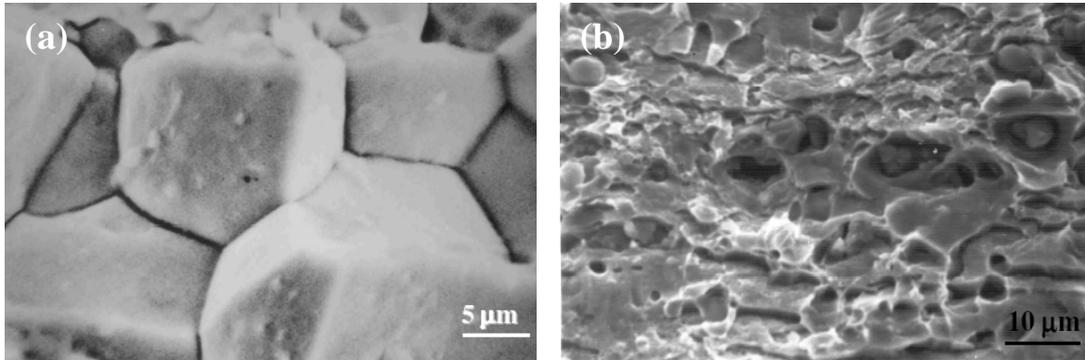
**Fig. 1.** SEM fractographs of 7010 Al-alloy in: (a) peak aged condition, shows typical intergranular cracking of recrystallized grains; and (b) over aged condition, shows predominant ductile fracture
