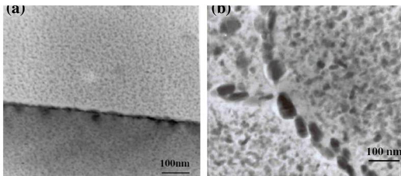
**Fig. 3.** TEM micrographs of 7010 Al-alloy in: (a) peak aged condition, shows fine precipitates in the matrix and continuous grain boundary precipitates ; and (b) over aged condition, shows coarse precipitates in the matrix and broken network of coarse grain boundary precipitates
