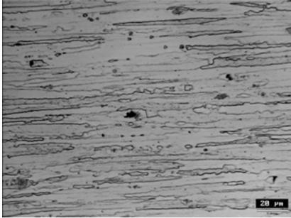
**Fig. 6.** Optical micrograph of 0.25 wt.% Sc containing 7010 Al-alloy in peak aged condition, shows fibrous non-recrystallized grains
