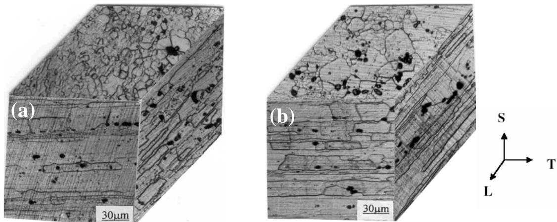
**Fig. 2.** Optical micrographs of 7010 Al-alloy in: (a) peak aged condition; and (b) over aged condition, shows elongated pancake shaped grains and equiaxed recrystallized grains along the long-transverse direction
