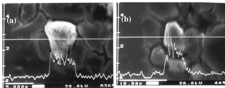
**Fig. 4.** SEM micrographs of 7010 Al alloy in: (a) peak aged condition and (b) over aged condition, show passive film break-down in the vicinity of spherical intermetallic particles, when exposed to 3.5% NaCl solution for 24 h (WDX Cu scans show the spherical intermetallic particles are rich in Cu)
