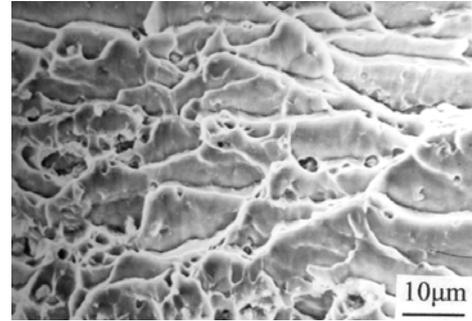
**Fig. 7.** SEM fractograph of 0.25 wt.% Sc containing 7010 Al-alloy shows a predominant ductile failure
