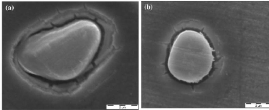
**Fig 5.** SEM micrograph of (a) peak aged (b) over aged, 7010 Al alloys exposed to 3.5% NaCl solution for 10h, shows no significant film break-down along the grain boundary
