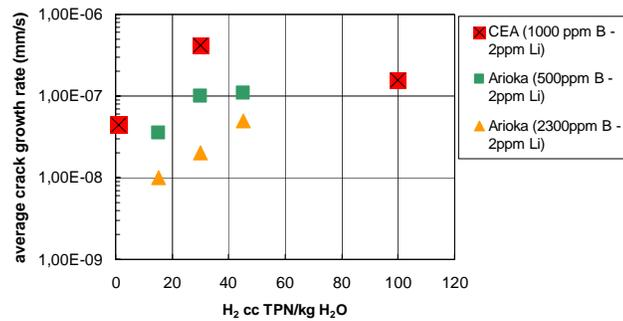
**Fig. 7.** Evolution of the measured average crack growth rate with respect to the dissolved hydrogen level – CERT tests on specimens cold-worked by shot-peening, comparison with results reported by Arioka [13]
