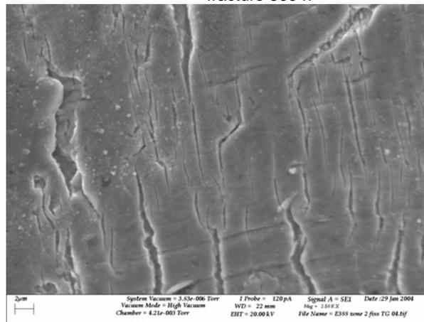
**Fig. 9.** Fracture surface showing an area of transgranular brittle fracture observed on a specimen previously cold-worked by cold rolling, pre-exposed during 2000h in hydrogenated primary water at 360°C and tensile tested ( $5 \times 10^{-8} \text{ s}^{-1}$ ) in primary water at 140°C
