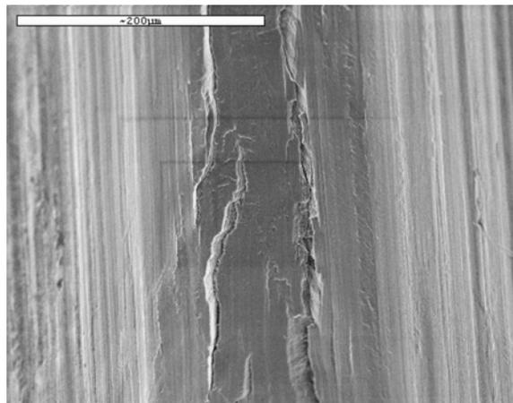
**Fig. 6.** Crack initiation observed inside the notch on a specimen initially cold-worked by fatigue and then tested under constant load (850 MPa); cross sections show that maximum crack depth is less than 20 µm, PWR primary water, 360°C, 17,000 h testing
