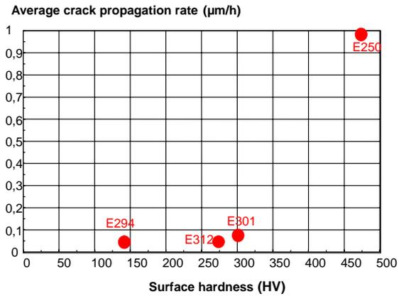
**Fig. 5.** Evolution of the average crack growth rate with respect to the initial surface hardness, cold-worked specimens (shot-peening) tested by CERT in primary water,  $1.5 \times 10^{-7} \text{ s}^{-1}$ , 360°C
