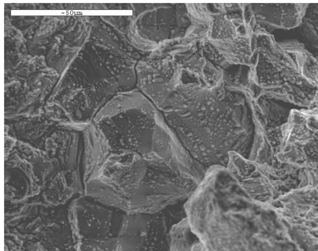
**Fig. 3.** Fracture surface obtained after CERT on a notched specimen (full annealing performed after machining of the notch); note the intergranular nature of SCC without cold-work, 304L, PWR primary water 360°C, time to fracture 2000 h
