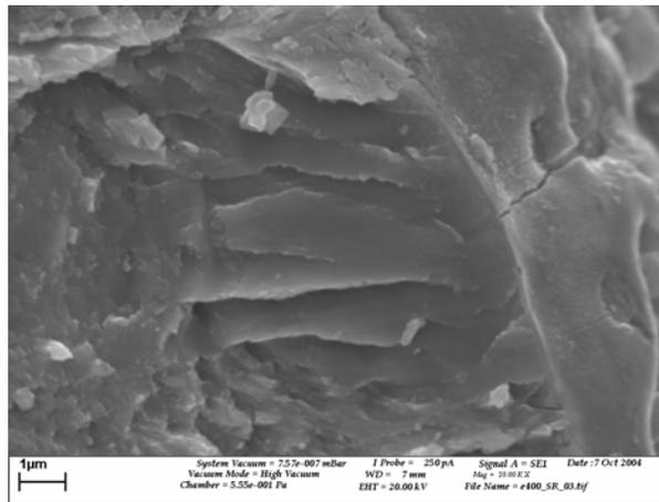
**Fig. 10.** Surface cracking observed on a specimen previously cold-worked by shot-peening, pre-exposed during 2000h in hydrogenated primary water at 320°C and tensile tested ( $5 \times 10^{-5} \text{ s}^{-1}$ ) in air at laboratory temperature
