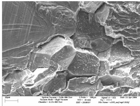
**Fig. 8.** Fracture surface of specimen previously cold-worked by shot-peening and tested by CERT ( $1.5 \times 10^{-7} \text{ s}^{-1}$ ), primary water at 320°C, hydrogen level 100 cc H<sub>2</sub>/kgH<sub>2</sub>O.STP, intergranular and transgranular fracture, time to fracture 500 h
