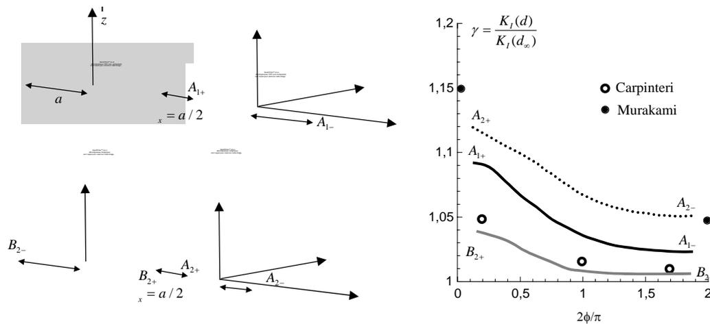
**Fig. 3.** Variation of the amplification factor  $\gamma$  along the crack front for two identical semi-circular coplanar cracks and for two different semi-circular coplanar cracks. The distance between the cracks is  $d = a/2$
