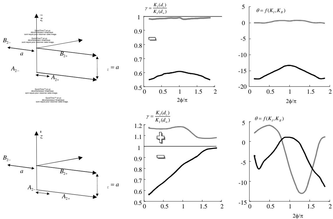
**Fig. 4.** Variation of the amplification factor  $\gamma$  and the deviation angle  $\theta$  along the crack front for two semi-circular stacked cracks in symmetric and non-symmetric configurations. The distance between the cracks is  $d_z = a$
