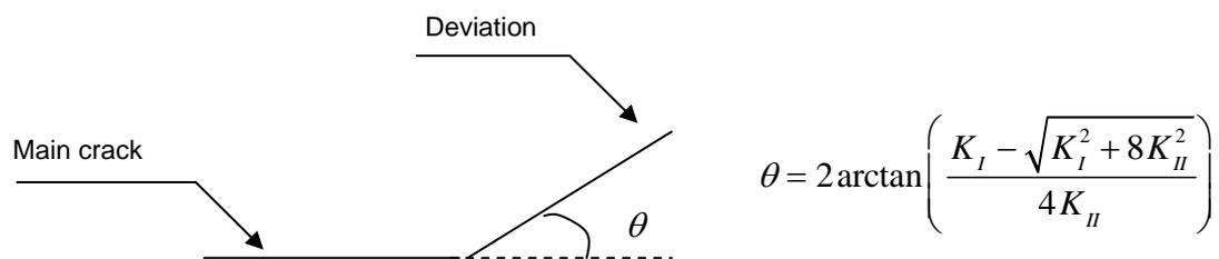
Fig. 2. Local direction of crack propagation
