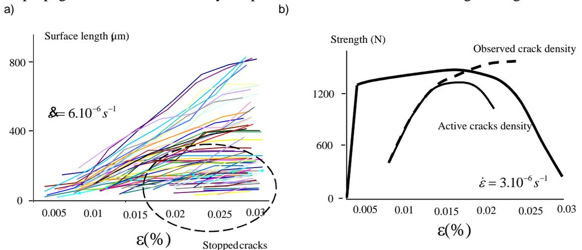
**Fig. 1.** Surface cracks distribution: a) length of all observed cracks and b) density of all observed cracks and density of active cracks (without stopped cracks)
