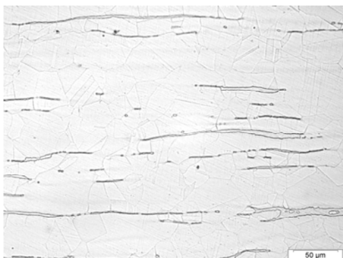
Fig.2. Microstructure at mid thickness on 304L SS
