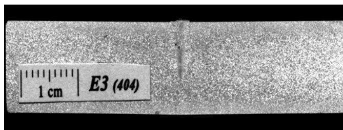
Fig. 6. The melting depth approximately 8 mm. The face is 3,5 mm wide. There are two little ball-like air sacs \phi 0,2 mm (2011) pursuant to PN-EN 30042:1994.
