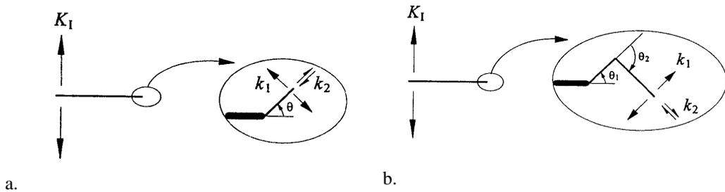
**Fig. 2.** Macrocrack with microcrack path deflections: a) simple kink with kink angle  $\theta$ , b) double kink with kink angle  $\theta_1$  and  $\theta_2$
