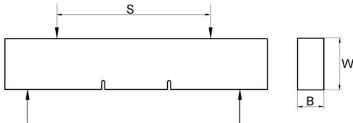
Fig. 4. The double-notched four-point bend test
