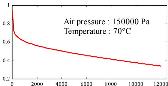
Fig. 3 : Graph showing the voltage [V] of a cell as a function of current density [A/m<sup>2</sup>] (polarisation curve)
