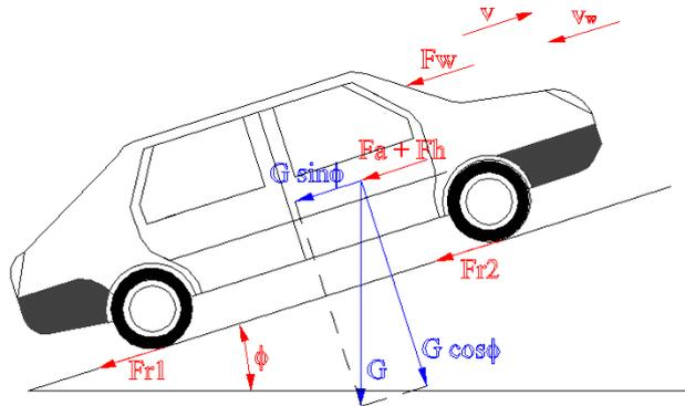
Fig. 1. Elementary forces acting on the vehicle
