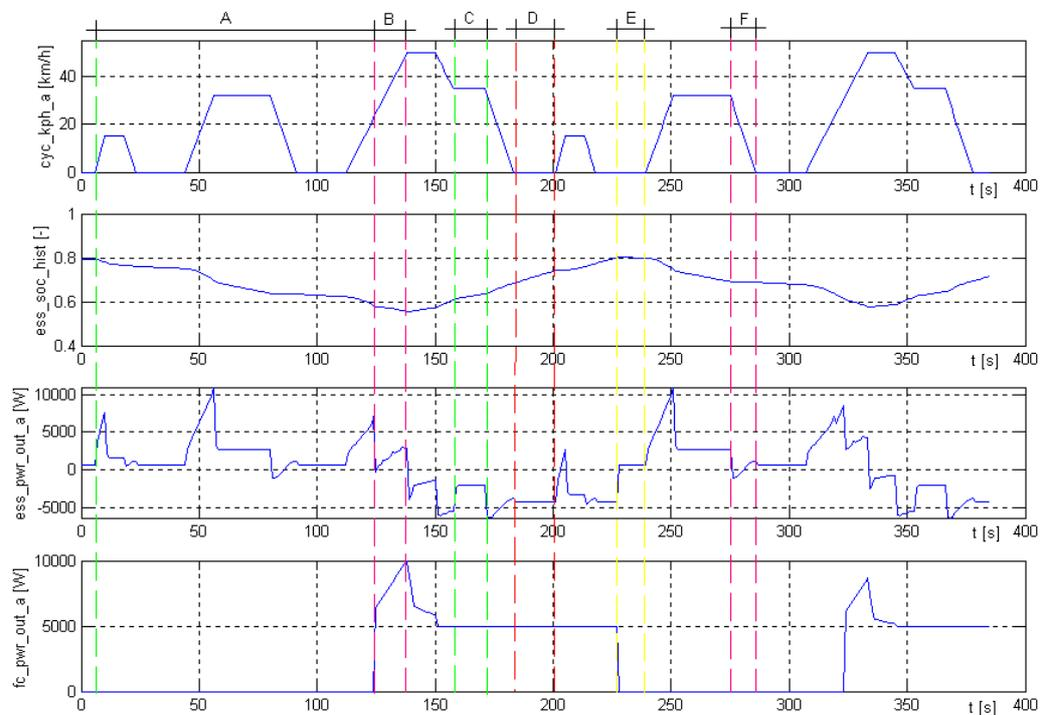
Fig. 5. Simulation transients at the double ECE cycle; cyc\_kph\_a - vehicle speed, ess\_soc\_hist - SC SOC, ess\_pwr\_out\_a - output power of SC bank, fc\_pwr\_out\_a - power available from the fuel cell converter
