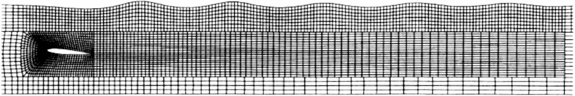
An example of application of the ITM method for the case of determination of the wave system on the free boundary generated by a hydrofoil moving under the surface (two-dimensional flow).
