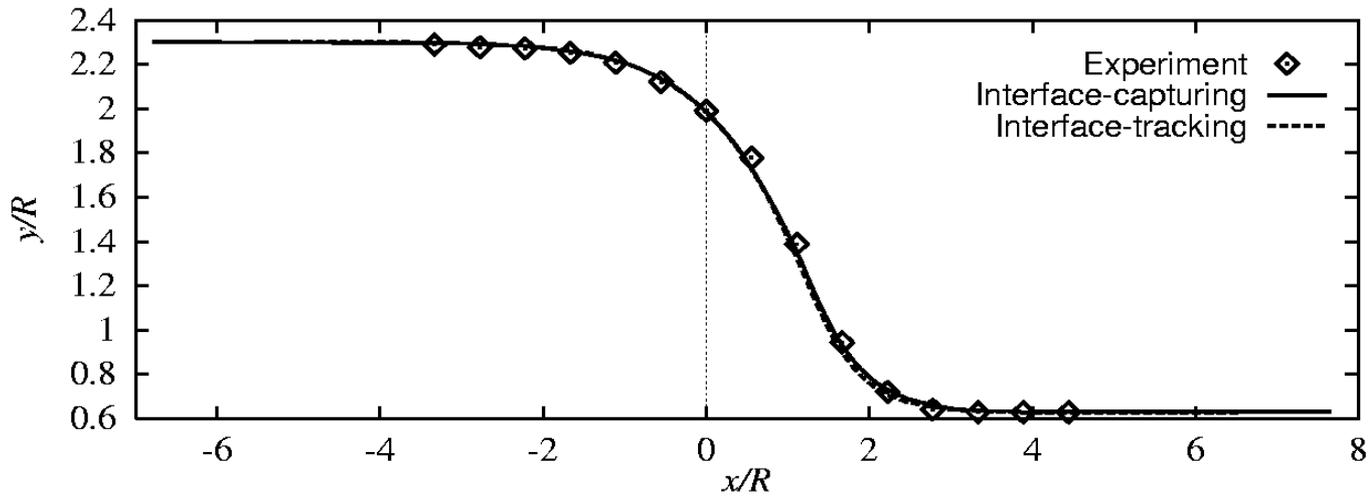
Supercritical free surface flow over a semi-cylindrical obstacle on the bottom
