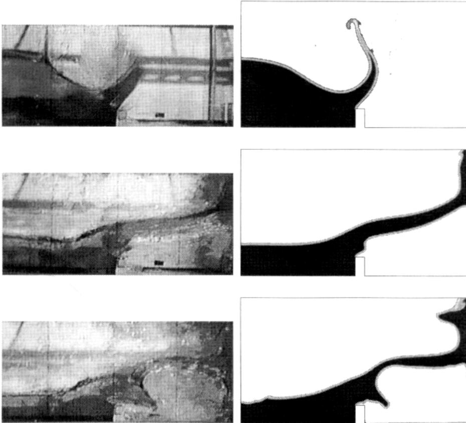
The consecutive phases of unsteady flow after sudden breaking of a barrier, calculated by the Volume of Fluid (VOF) method, using „one fluid approach”, in comparison with experiment.
