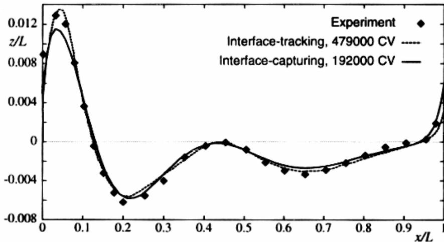
Comparison of the experimentally observed and calculated wave profile along the ship hull
