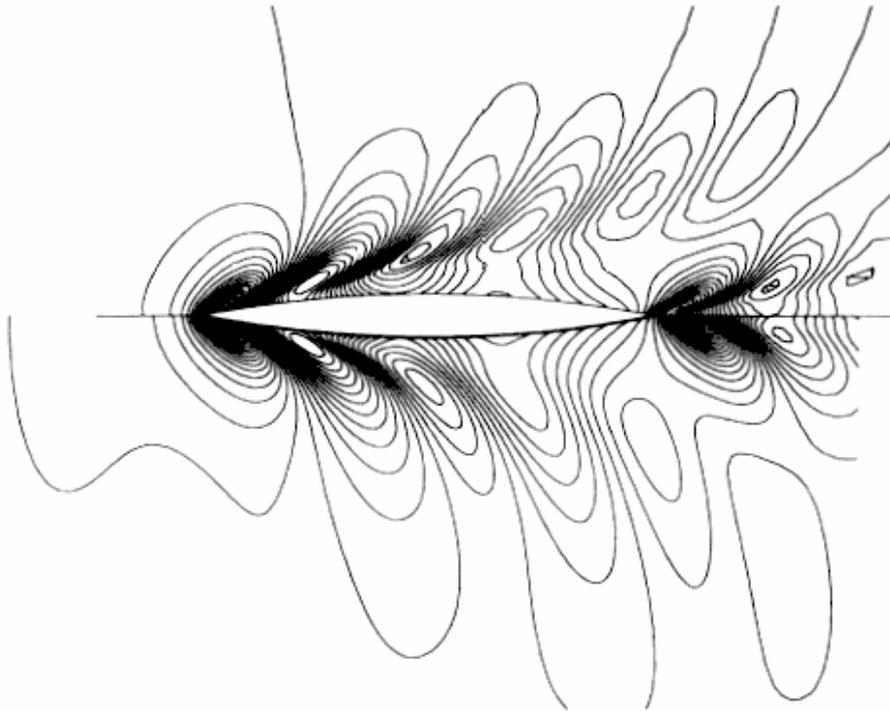
Calculated map of the wave system – upper part of the picture – VOF method, lower part of the picture – ITF method
