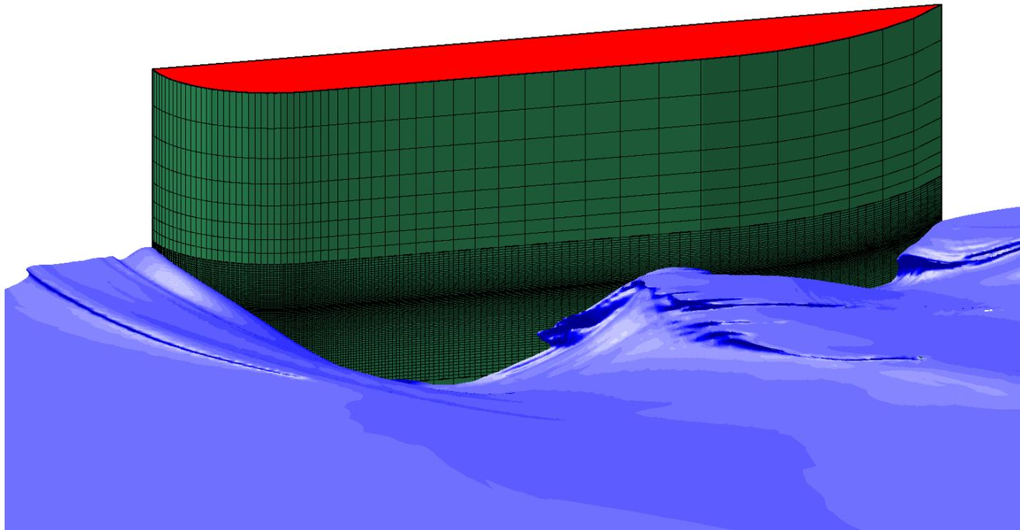
Free surface flow around a blunt ship hull
