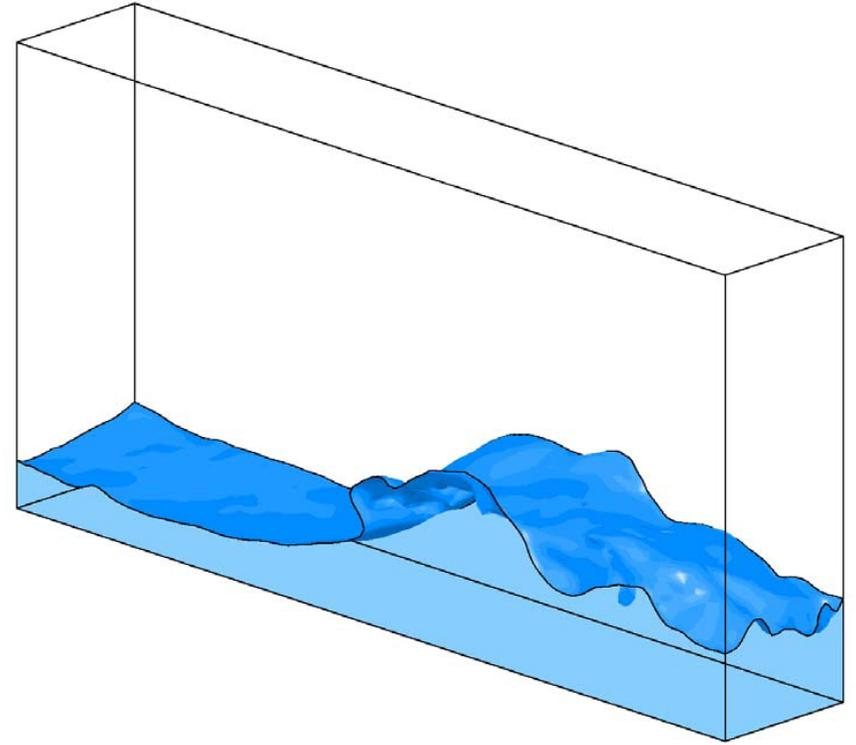
Calculated phenomenon of liquid sloshing in the tank swaying horizontally
