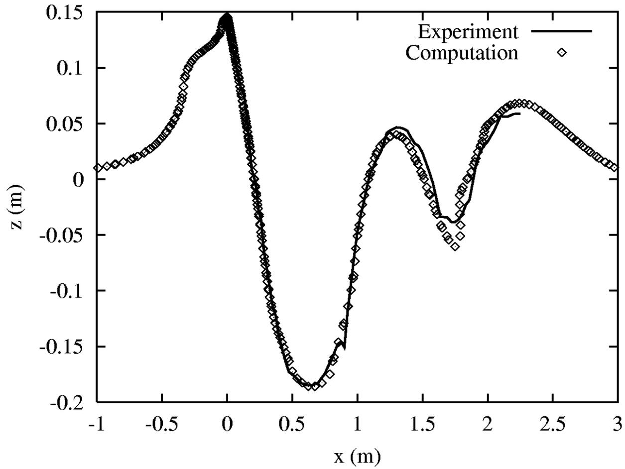
Comparison of observed and calculated free surface level along the blunt ship hull
