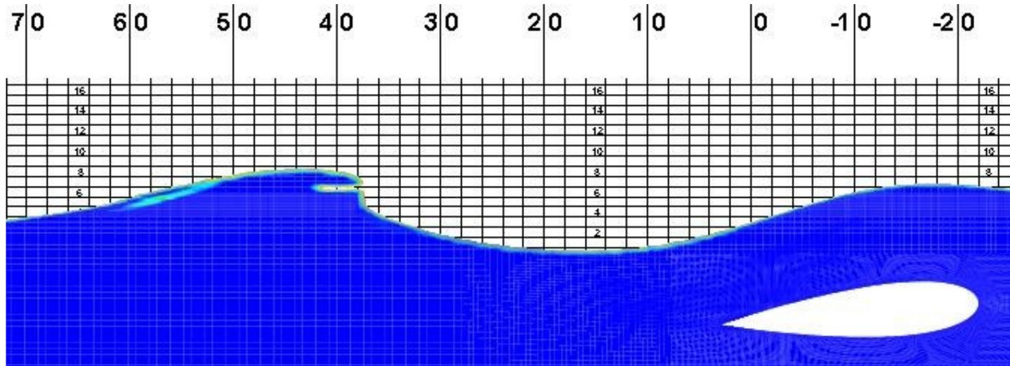
Free surface deformation over the moving submerged hydrofoil
