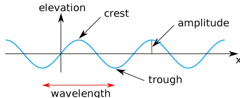
The simplest two-dimensional model of surface waves is the Airy's theory
