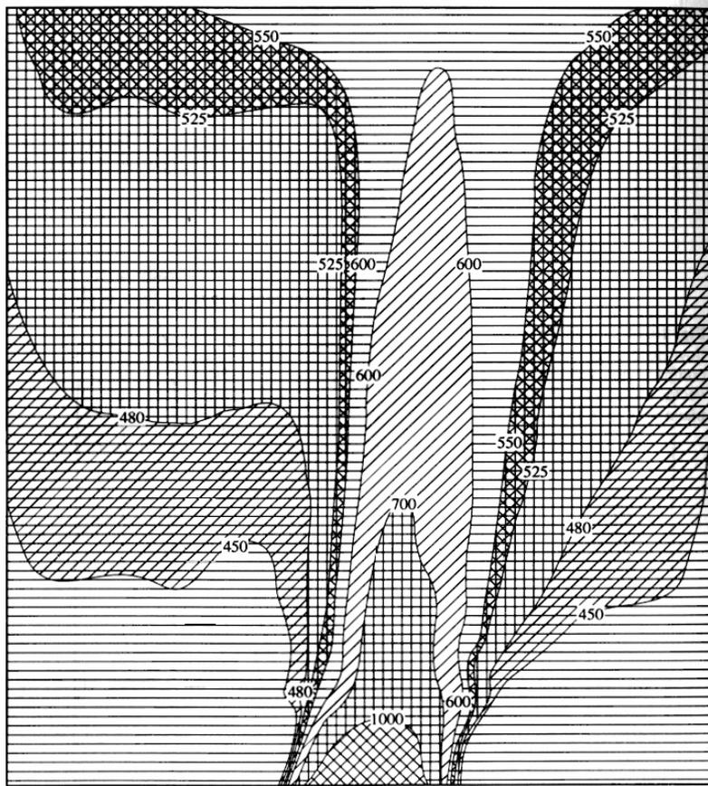
← The calculated temperature field in the section z-y for  $x=3,00$  [m]
