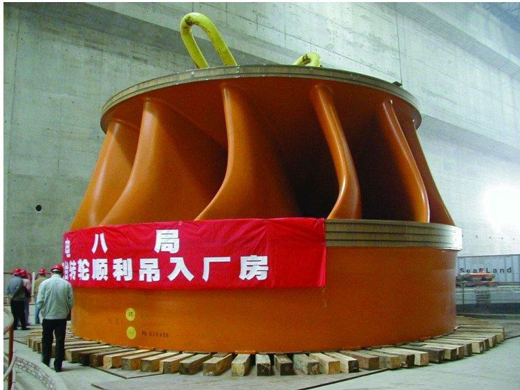
Rotor of the Francis water turbine
