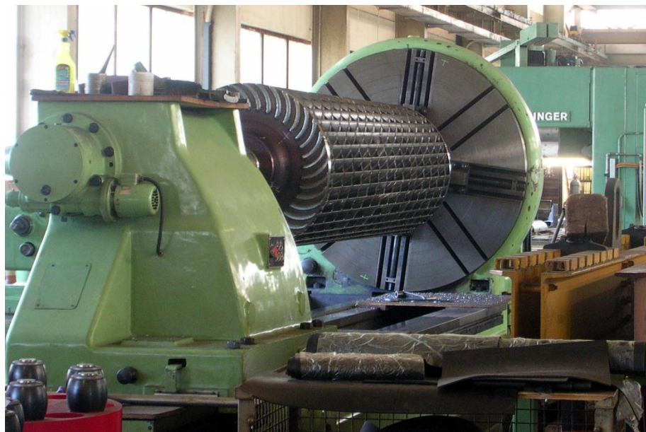
Rotor of a diagonal (mixed flow) pump
