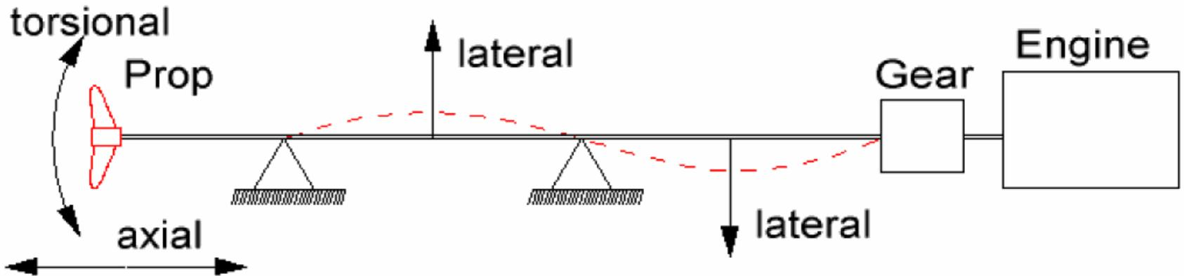
Scheme of a ship propulsion system. The most important are the torsional and longitudinal (axial) vibrations. An important component of the system is the propeller, being a heavy object immersed in water. Variable hydrodynamic forces are generated on the propeller, constituting the main source of vibration excitation.
