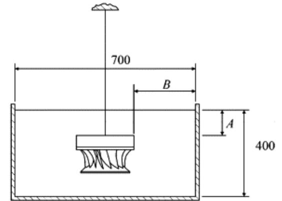
Test set-up for measurements in water and in air
