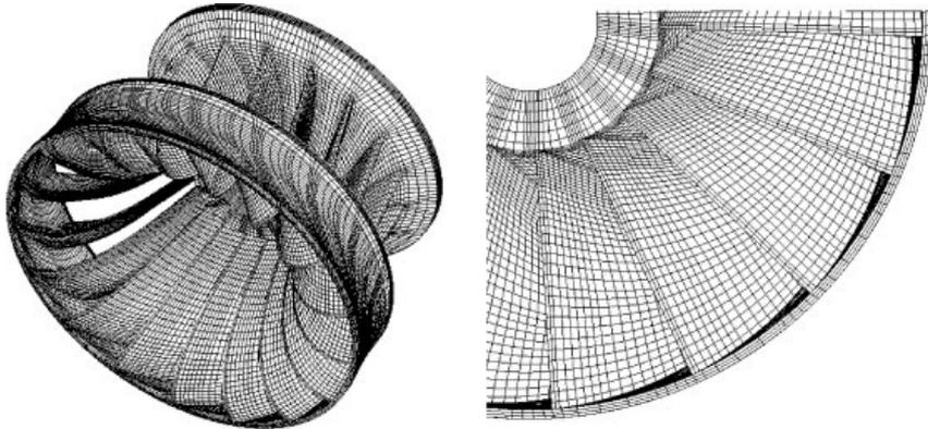
Every geometrically repeatable sector of the rotor was modelled by 6133 hexahedral finite elements. The results of calculations were compared with experimental measurements discussed before. In all cases the immersion in water has reduced the own frequencies of vibration of the rotor.
