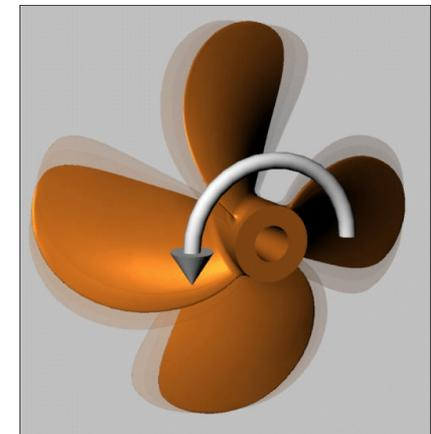
Determination of the entrained mass for the propeller is necessary for correct analysis of vibration of the ship propulsion system. There are many methods for determination of the entrained mass. The simplest are the empirical formulae:
