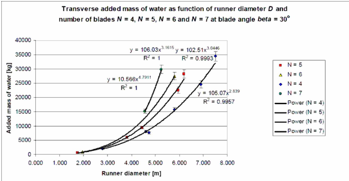
The entrained mass  $M_{22}$  for rotors of different diameters and numbers of blades at the same pitch setting angle  $\beta$
