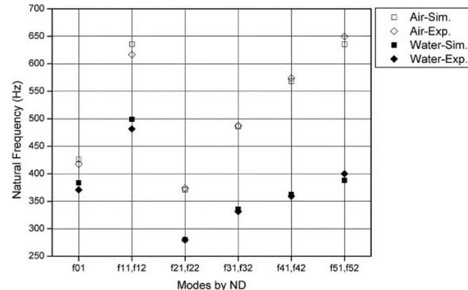
Comparison of the calculated and measured frequencies of the different vibration modes in air and in water
