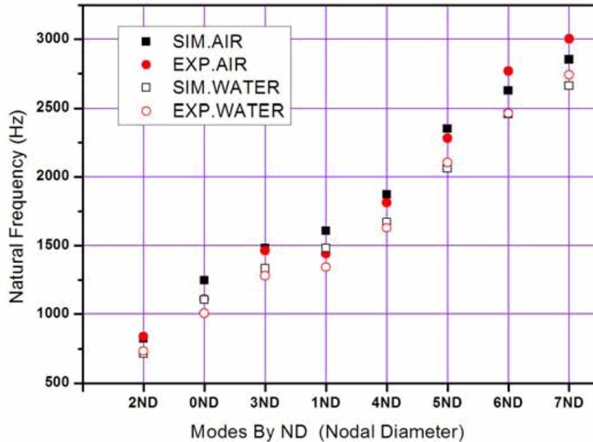
Comparison of the calculated (SIM) and measured (EXP) own vibration frequencies of the rotor in air and in water
