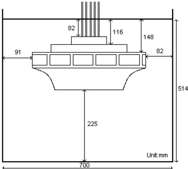
Model of the rotor of a reversible machine (pump-turbine) has been tested in air and in water. Model vibration was excited by an inducer in 384 points shown in the picture. The responses for several own modes of vibration were registered.
