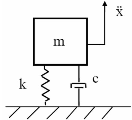
The entrained mass increases the inertia of the object, thus it counteracts oscillations. In this case the equation describing oscillations has the form:
