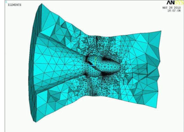
Rotor model in the Finite Element Method
