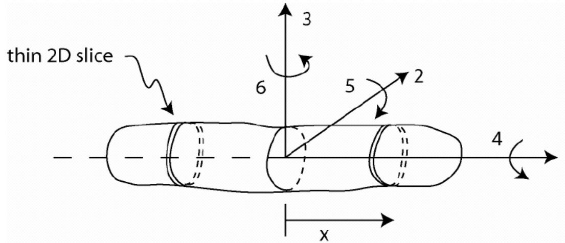
In this theory the object may be cut into „slices” and the entrained mass coefficients for two-dimensional sections may be integrated along the object:
