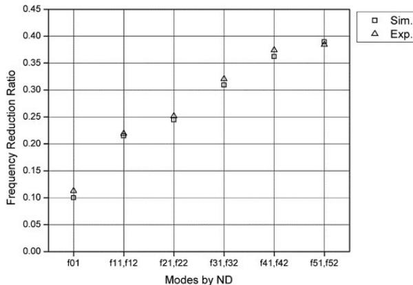
Measured and calculated degree of reduction of frequency of the different vibration modes in water
