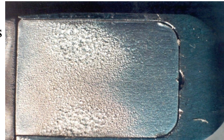
Aluminum sample after the erosion test
