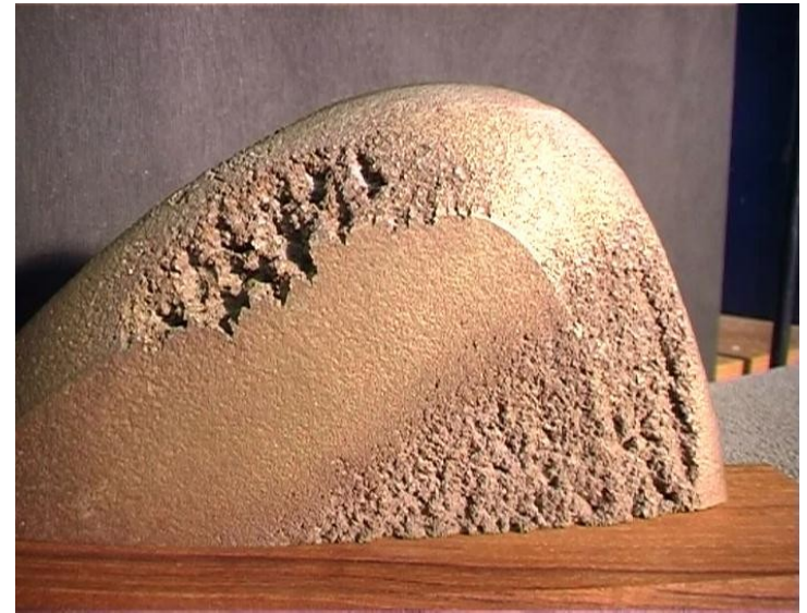
A piece of heavily damaged marine propeller blade
