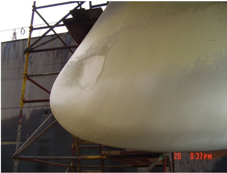
Initial phase of erosion on the marine propeller blade
