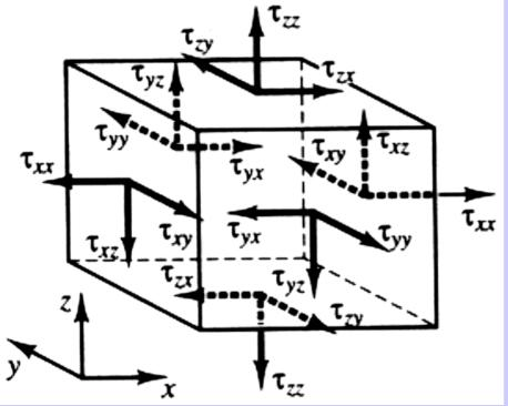
The above relations describe the normal and shearing viscous stresses as shown in the picture. As these relations link the stress field to the velocity field, their substitution to the momentum conservation equation reduces the number of unknowns. This is demonstrated in the next lecture.
