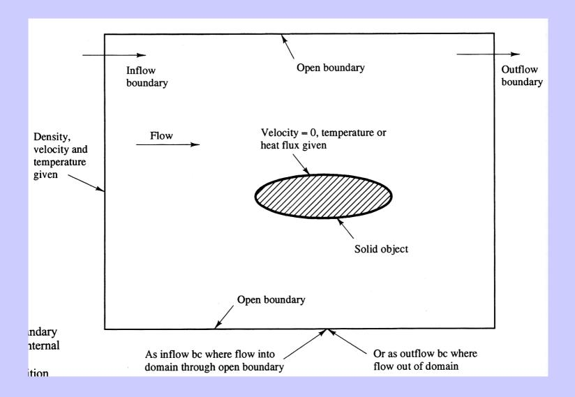
Scheme of the boundary conditions for an external flow
