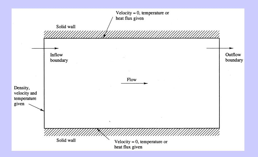
Scheme of the boundary conditions for an internal flow
