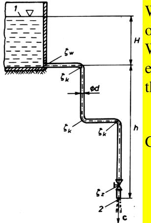
Water flows from an open tank through a pipe of length l=200 [m] and diameter d=100 [mm]. What should be the water level H in the tank to ensure the volumetric intensity of outflow from the pipe equal to Q=40 [l/s]?
