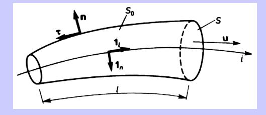
The flow of fluid in a closed channel is described by means of the simplified model of a one-dimensional flow. It is assumed that the axis of the channel is "almost" a straight line and the flow across the section S takes place with a "representative" velocity  $\tilde{u}$ , that is some mean velocity.
