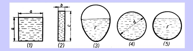
In the case of non-circular or partly filled channels the important parameter is so called hydraulic radius, or the ratio of the fluid stream cross-section area to the wetted circumference:
