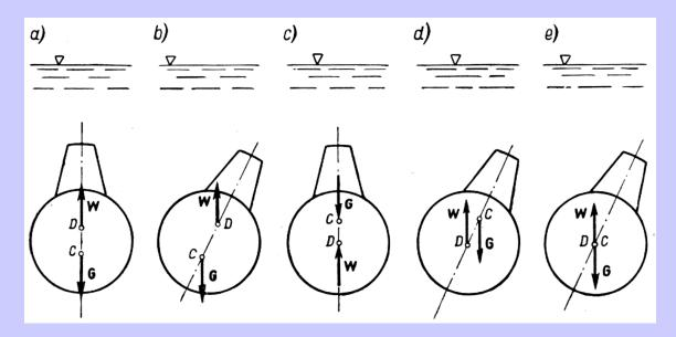
**Stable equilibrium** – Centre of buoyancy is located above the centre of gravity – Figs a) and b). Deflection from the equilibrium position generates the moment of the pair of forces acting against the deflection and enforcing return to the previous position.
