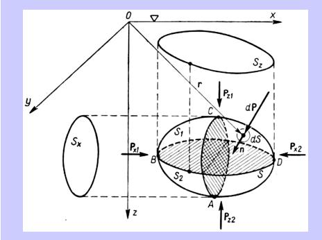
The horizontal components of the hydrostatic force are equal zero. The total hydrostatic force is reduced to the vertical force acting on two parts of the suface joined at the common contour: the lower part BAD and the upper part BCD. Force at the lower surface
