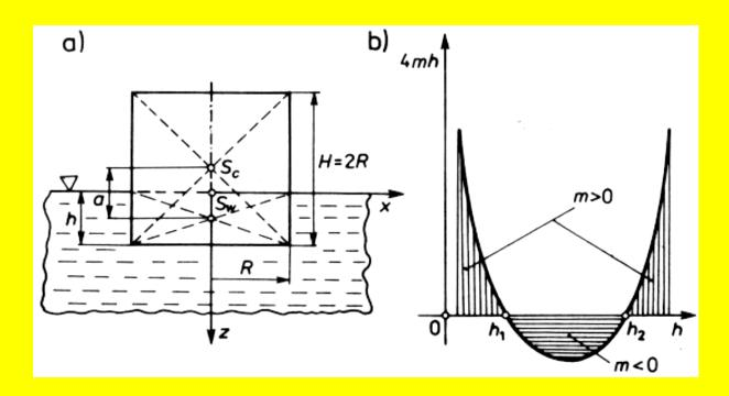
A circular cylinder having the base radius *R* and height H=2Rfloats in an upright position (Fig. a). The centre of gravity of the cylinder coincides with its geometrical centre. For which submergence of the cylinder *h* its equilibrium is stable? The waterline of the cylinder is a circle, the inertia moment of which is:
