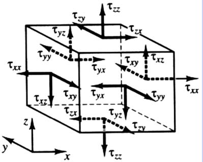
The unknowns in the momentum conservation equations are: pressure, velocity components and stresses representing the surface viscous forces. Even after adding the mass conservation equation to the system, the number of unknowns is greater than the number of equations. In order to reduce the number of unknowns and close the system an appropriate fluid model must be introduced.
