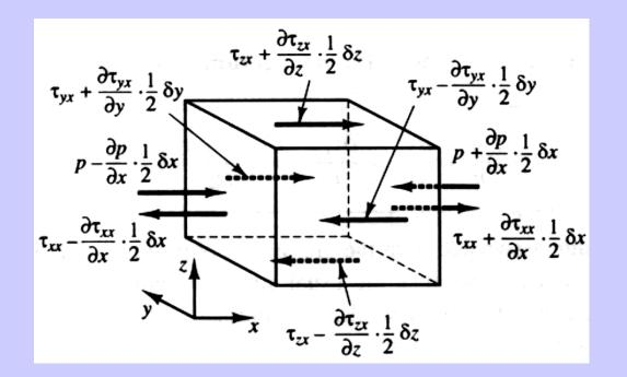
Forces acting on the element walls perpendicular to the x direction
