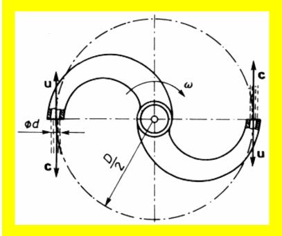
The Segner wheel of diameter D is supplied with water having the flow intensity Q. Disregarding the frictional losses and flow losses determine the angular velocity of the wheel rotation  $\omega$ . Assume the outlet diameter of the nozzles equal to d. Assume that the resultant moment on the wheel is zero. The Segner wheel rotates in the direction opposite to the water outflow, hence the absolute outflow velocity c is:
