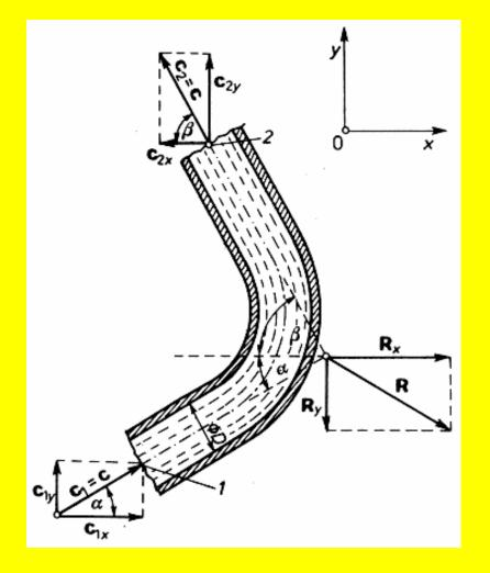
Water flows through the bent pipe of diameter D=80 [mm] with flow intensity Q=0.08 [m\*\*3/s]. **Disregarding the losses, calculate** the force exerted by the water stream on the pipe. The inlet part of the pipe is located at the angle  $\alpha = \pi/6$  to the horizon, while the outlet part is located at the angle  $\pi/3$ . In both inlet and outlet crosssections of the pipe the pressure is equal to the ambient pressure pb.
