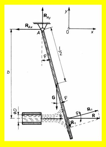
The stream of perfect liquid of density **ρ flows out of the nozzle and hits the** ideally smooth plate of weight G and length l. The plate can rotate around the bearing A located at the distance b from the nozzle axis. Knowing that the intensity of the outflowing stream is Q, and the nozzle diameter is D, calculate the components of the reaction in the bearing and the angle  $\varphi$  of inclination of the plate in the state of equilibrium.
