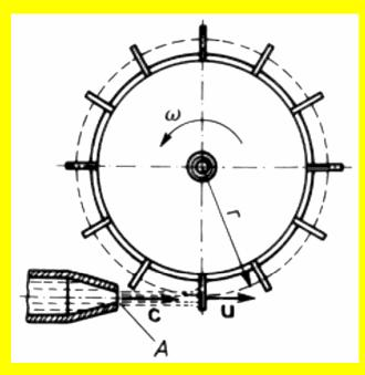
The stream of water of intensity q=0.01 [m\*\*3/s] flows out of the nozzle and hits the flat blades of the water wheel with the mean radius r=1.0 [m]. **Disregarding the losses, calculate the** effective power and the efficiency of the wheel, if its angular velocity is equal to  $\omega = 5.0$  [1/s], and the crosssection area of the duct is equal to A=500 [mm<sup>\*\*</sup>2]. For what angular velocity of the wheel the effective power reaches the highest value?
