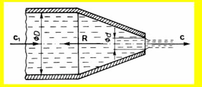
Water is ejected with the mean velocity c=15 [m/s] from the nozzle of diameters D=80 [mm] i d=20 [mm]. Disregarding the pressure difference calculate the hydrodynamic reaction force exerted by the water stream on the duct.
