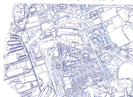
Step 2: Import map into vector illustration software. Surveyed maps are generally supplied in many layers and some layers may need switching off. Do not delete the layers as they may be required for reference later.
